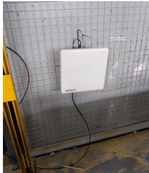
Figure 4. One of the RFID Antennas temporarily installed for data collection in the factory of a Brazilian company.
