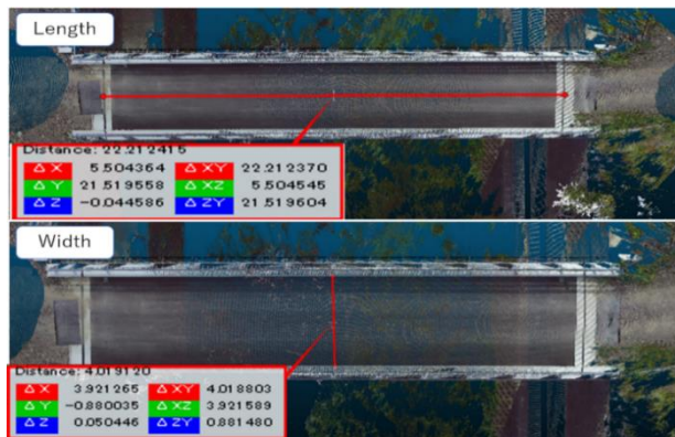
Figure 9. Length and width based on the combined point cloud data for Warazuhata Bridge
