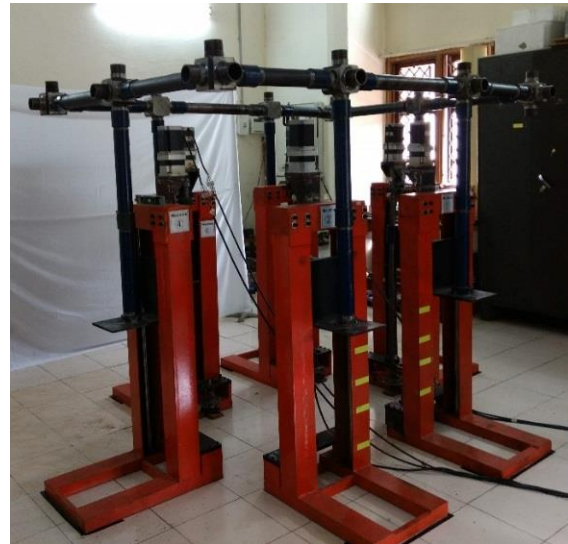
Figure 1. The partially constructed structural frame on the automation system
