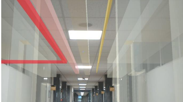
Figure 13. Verification of BIM-MEP model visualization through MR device
