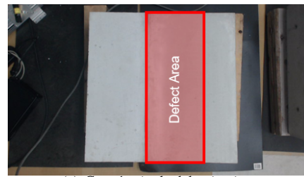
(a) Case 1: single delamination.
