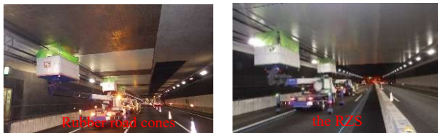
Figure 7. Demonstration Experiment (Left: rubber road cones Right: the RZS)
