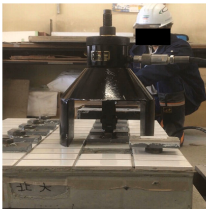
Figure 9. Tile removal operation. Nuts are installed on the tiles to be removed.
