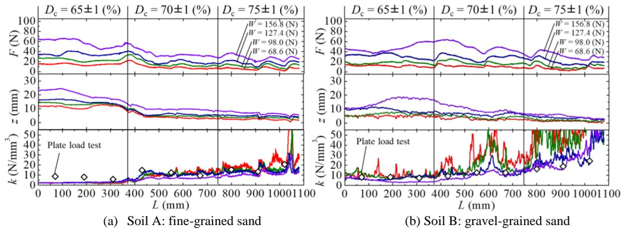
Figure 6. Experiment results and estimated subgrade reaction modulus
