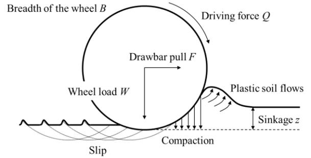
Figure 2. Soil-wheel interaction
