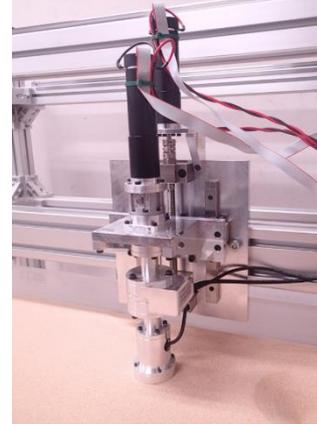
Figure 4. Small-diameter plate load test equipment
