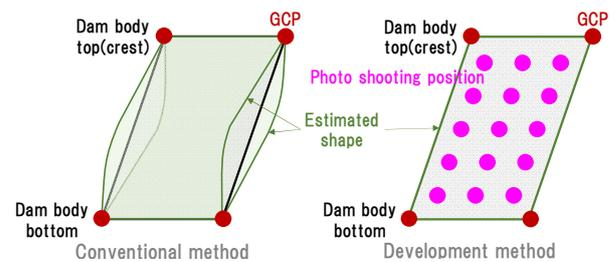
Figure 5. Improving the accuracy of the three-dimensional modeling
