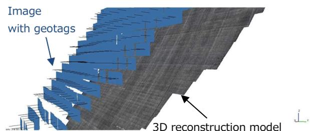
Figure 12. An example of the photograph's alignment (Dam-2).
