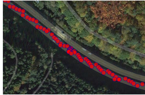
Figure 3. Visualization of the reversing points close to the paver from a real world example.
