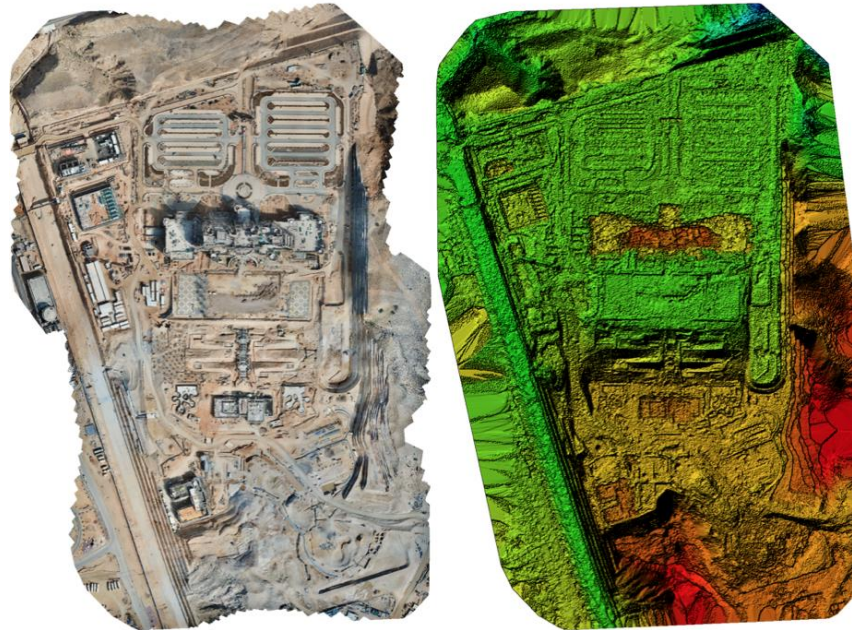
Figure 4. Orthomosaic Model of Construction Plot
