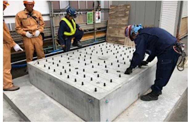
Figure 3. Concrete specimen and marking work
