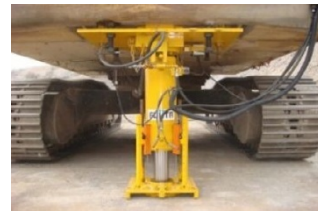
Figure 9. Measuring machine of a remote control type bearing power of ground
