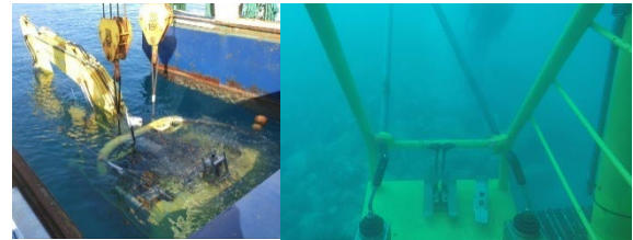
Figure 8. Captures of sea experiments (left figure; Excavator craned into the sea, right figure; Excavator working without divers on cockpit)
