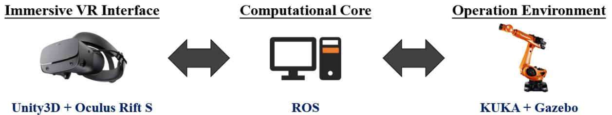
Figure 1. Collaborative human-robot construction system overview
