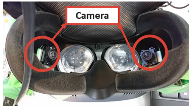
Figure 4. Two cameras installed inside the head-mounted display
