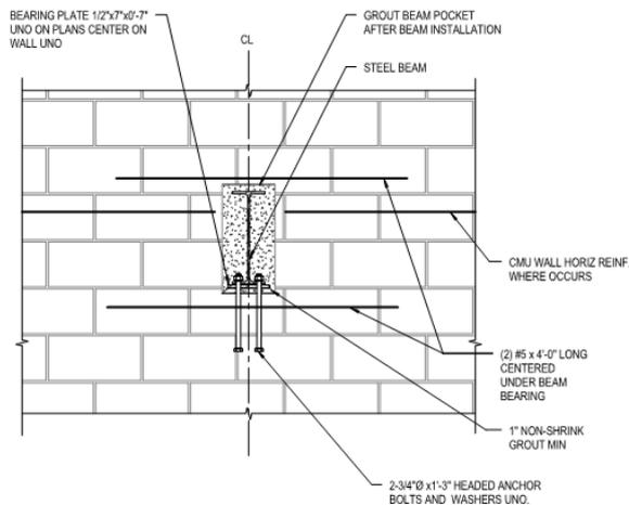
Figure 2. Bearing steel embeds on Concrete Masonry Wall.
