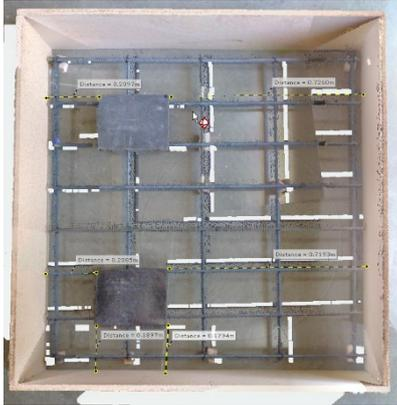
Figure 6. New layout with steel embed plates shifted to the left (as-built 2).
