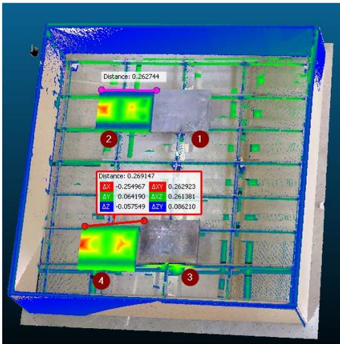
Figure 9. Determination of how far the embeds moved.
