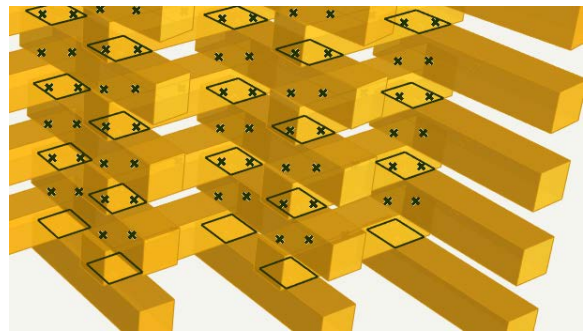
Figure 4. Geometry nailing points and gluing range
