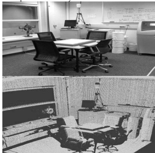
Figure 4. Photo image (top) and scanned point clouds image (bottom) for a lab meeting area
