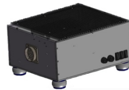
Figure 3. Excavator attribute-sensing module.
