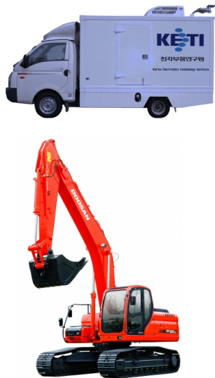
Figure 1. RCS and the electrohydraulic-driven excavator (plant).
