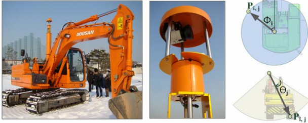
Fig. 1 3D laser scanner module of IES
