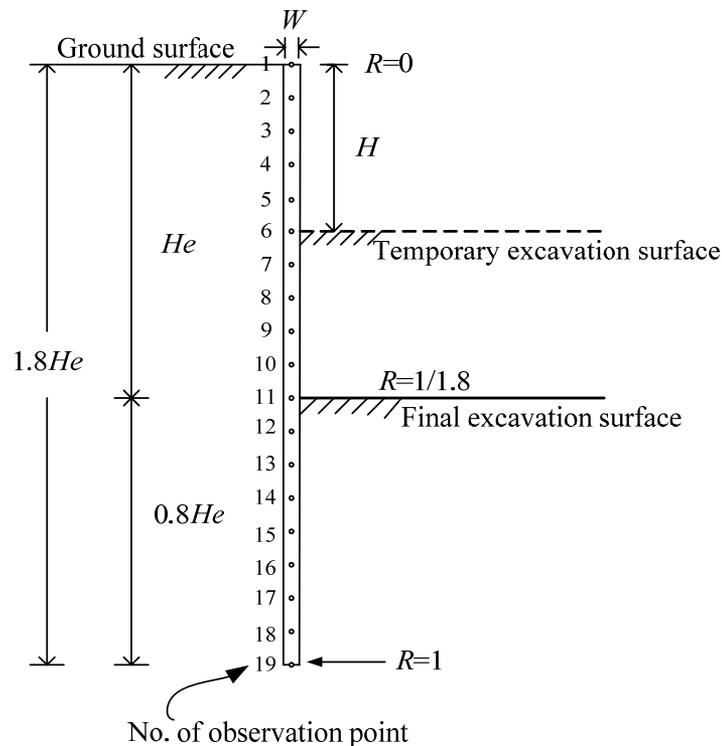
Figure 2. Representation of the Diaphragm Wall Structure
