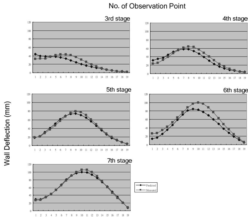
Figure 4. Wall Deflection Prediction Using the Modified Process
