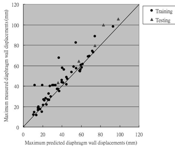
Figure 3. Measured vs. Predicted Maximum Diaphragm Wall Displacements.
