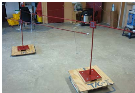
Fig. 1 Two T-type tower crane models for experiment
