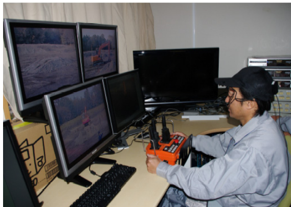
Photo 4 Operation using the remote controlled system
