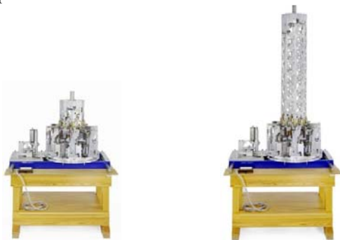
Fig. 02: HT1 scale model, retracted (left) and extended (right). K. Zuses first approach concerning the design of an auto-extendable and -retractable tower construction.
