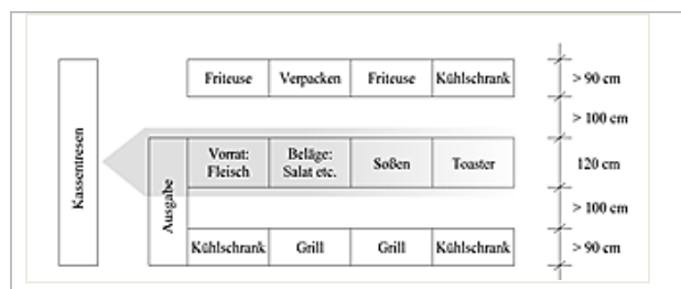
Fig. 3 Mc-Donalds kitchen: functional system for efficient processes.
