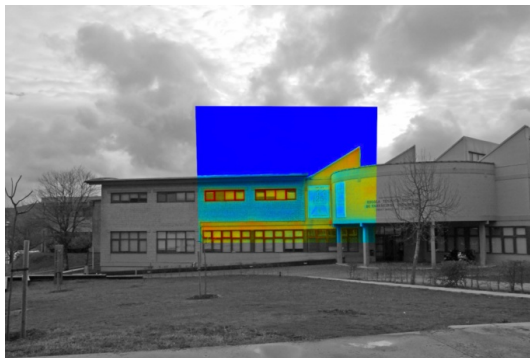
Fig. 4 Fused image, resulting from the fusion of visible and thermographic images in fig. 1 with and IHS fusion algorithm.
