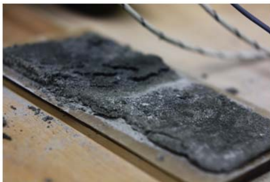
Fig 7 Failure of Continued Landing Pad
