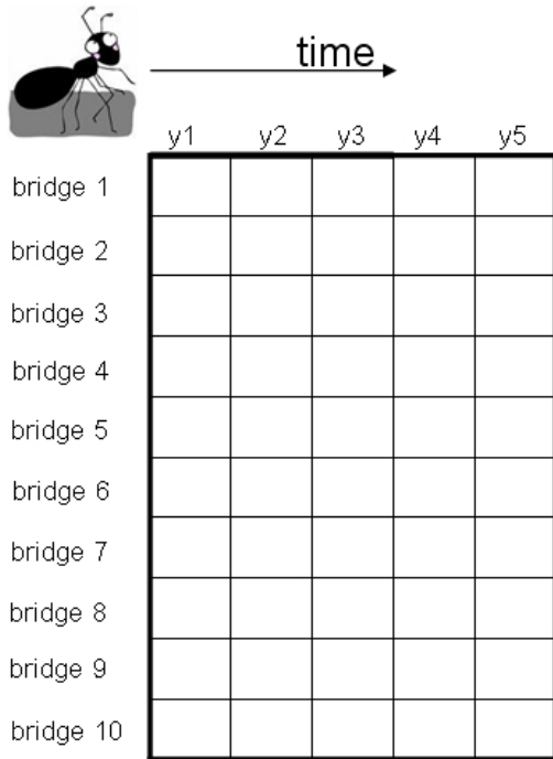
Fig. 2 Problem for 10 bridges and a schedule for five years modeled as a matrix
