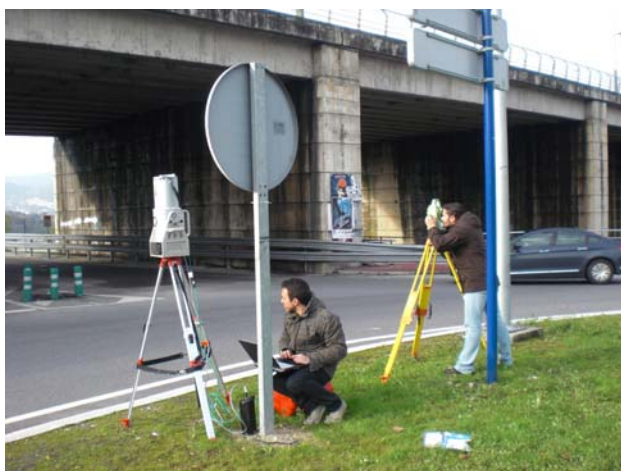
Fig. 3. RIEGL LMS Z390i during surveying process.
