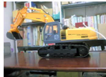
Motion 3: Curl bucket in as extracting stick while lowering boom a bit, and subsequently raising boom a bit
