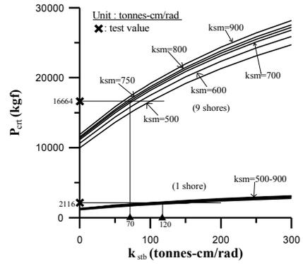
Figure 5 End Stiffness of Metal Post-Shores
