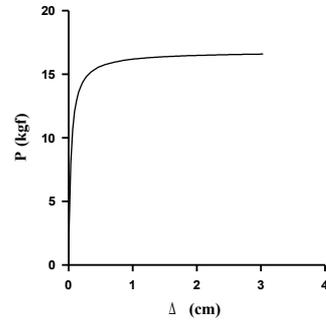
Figure 6(b) P-Δ Curve of 9 Metal Shoring System
