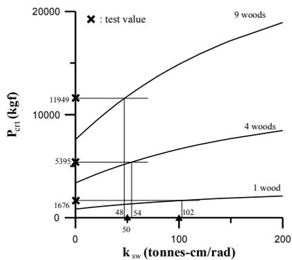
Figure 4 End Stiffness of Wood Post-Shores
