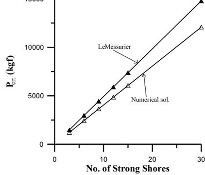
Figure 10 Critical Loads of Wood Shoring Systems vs. Leaning Columns (1 Strong Shore)
