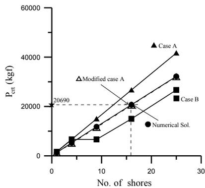
Figure 7 Critical Loads of Wood Shoring Systems
