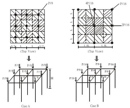
Figure 2 Arrangement of Load Case A and B
