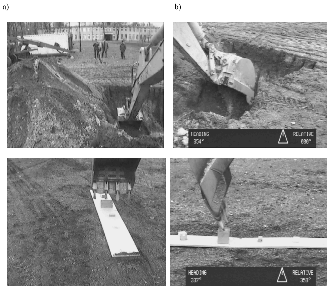
Fig. 3. A sight of picture set: a) camera (K3) placed beyond machine, b) cameras (K1 and K2) placed on a machine, c) monitor with a working equipment picture
