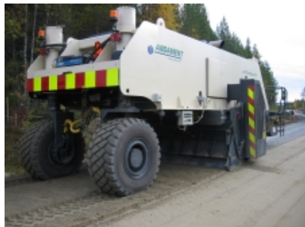
Figure 4. The first milling machine in Finland which has been equipped with an automated machine control system.
