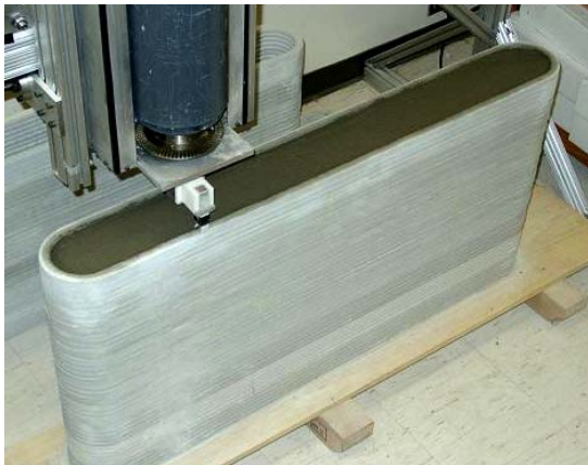
Figure 10. A concrete wall made by CC machine
