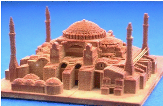
Figure 1. A complex geometry (Hagia Sophia in Istanbul) fabricated by a RP process [Source: MIT 3DP Laboratory]
