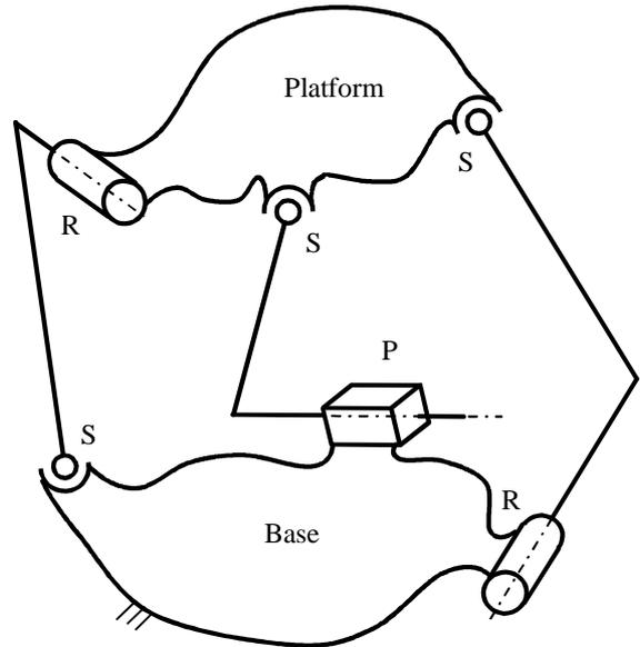
Fig. 2: Structure with topology SR-PS-RS (R, P and S stand for revolute, prismatic and spherical pairs, respectively)
