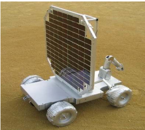
Fig. 1(b). Lunar rover to explore the presence of ice in the lunar polar region
