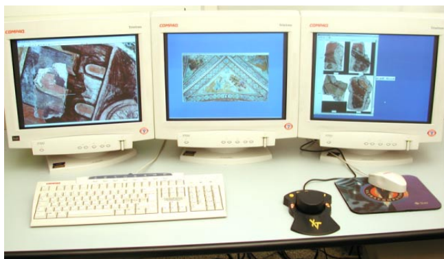
Fig. 3. The workstation for the virtual aided recomposition. From the left: the working area on which the images of fragments are moved while searching for their place; a scaled version of the whole fresco used for selecting the area of interest; one of the virtual containers used to organize fragments. A special mouse allows to rotate and translate simultaneously the fragments images on the working area.
