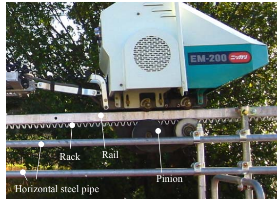
Fig. 1. Rack and pinion mechanism
