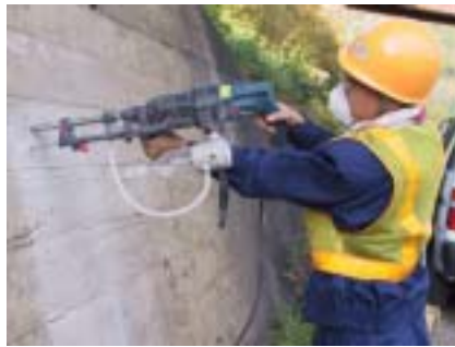
Fig. 6 Investigation of chloride content and carbonation depth by drilling method
