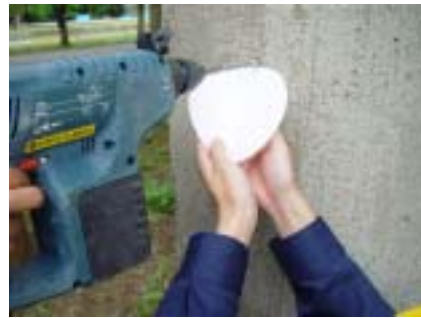
Fig. 6 Investigation of chloride content and carbonation depth by drilling method
