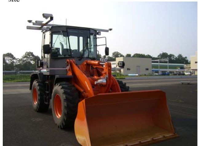
Fig.18 Sensors on YZ-4
