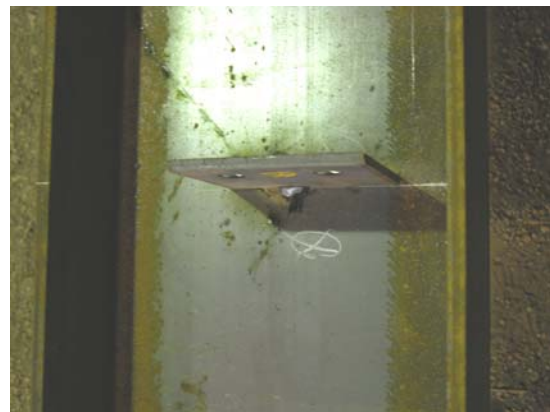
Figure 1. Component tack-welded in place. Note Fitter's locating marks.
