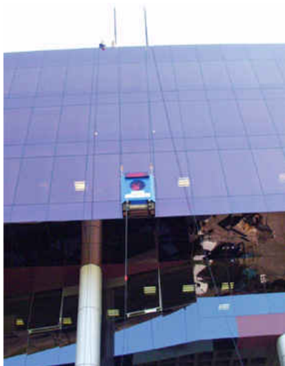
Figure 4. TITO – Automatic Façade Cleaning System ( CSIC )
