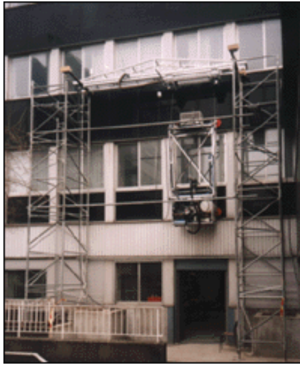
Figure 2. ARCOW Façade Cleaning System (Newcastle University; OCS Group; Cradle Runways)
