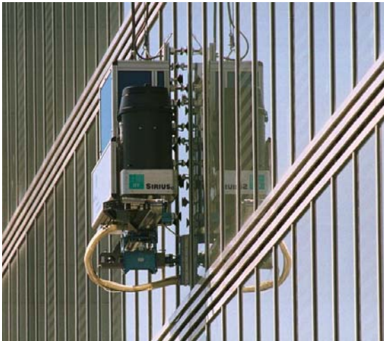
Figure 3. SIRIUSC – Automatic Façade Cleaning System ( Fraunhofer FhG, Dornier Technologie )
