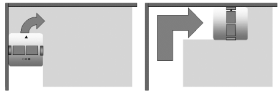
(b) Novel turning strategy, which enables to clean a corner Fig. 3 Overview of small-size window cleaning robot
