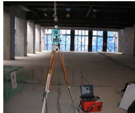
Figure 3 CCD camera mounted on non-prism total-station for taking photo images with 3D geometrical data
