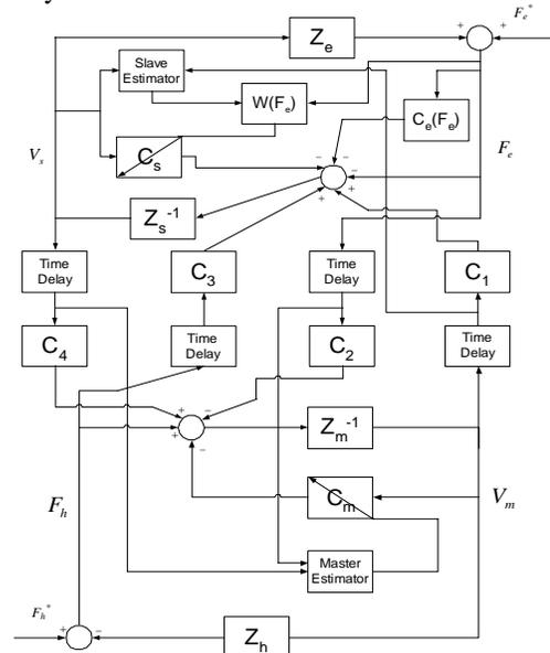
Fig. 3 the proposed bilateral teleoperation system block diagram
