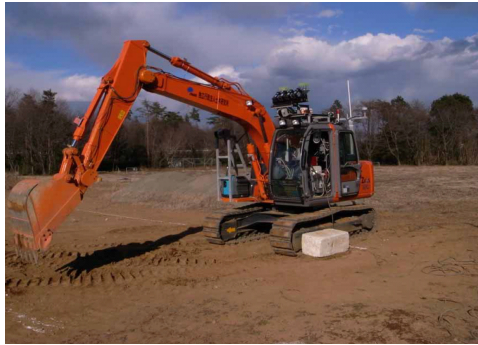
Figure.1 The hydraulic excavator to which remote control systems are attached
