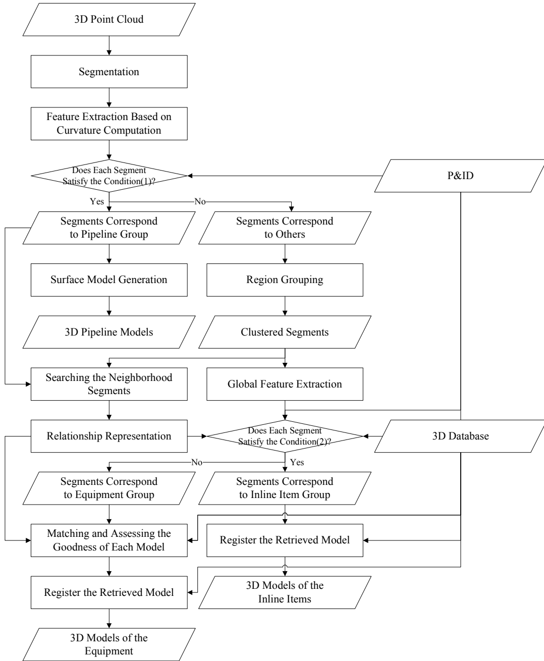
Figure 1 – Proposed knowledge-based approach for 3D reconstruction of as-built industrial plant models
