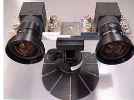
Figure 2 - Experimental prototype of stereo vision camera
