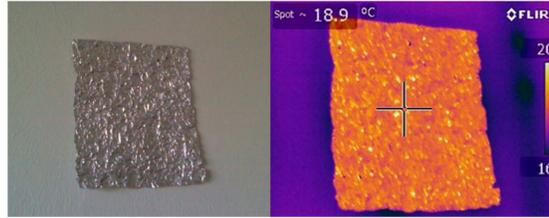
Figure 4 – Measuring the reflected apparent temperature with the crumbled foil
