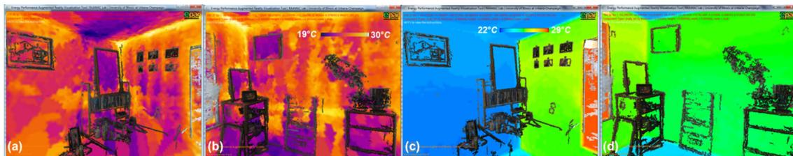
Figure 5 – 3D mesh based actual and simulated thermal performance along with the 3D building geometrical point cloud in EPAR models
