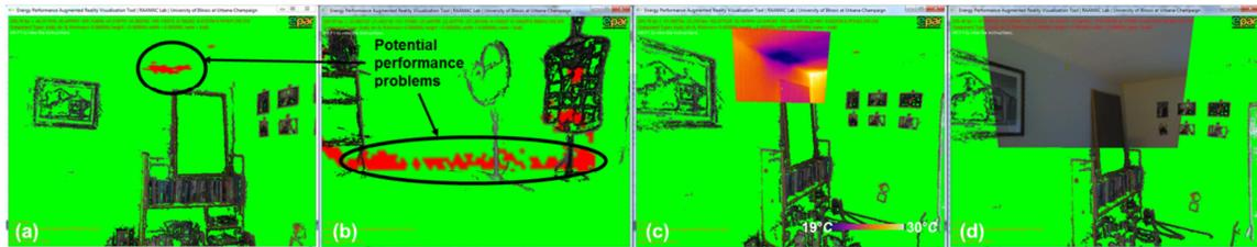
Figure 6 – Examples of the detected potential performance problems along with the 3D building geometrical point cloud and 3D-registered images within the EPAR models
